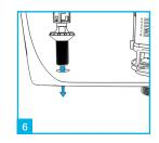
Place the valve in the correct position inside the cistern ensuring the conical rubber seal sits evenly inside the hole.
