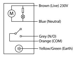
The auxiliary switch can be used as an interlock facility, thereby ensuring any auxiliary equipment is switched OFF when the valve is in the closed position. When the valve is in the fully open position the auxiliary equipment will be switched ON.\*
