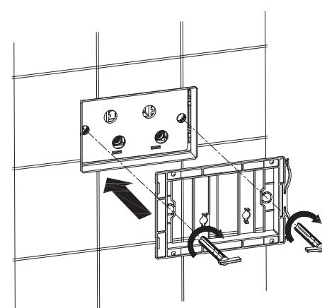
Fix the flush plate mounting bracket
