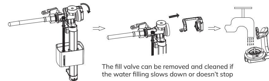
The fill valve can be removed and cleaned if the water filling slows down or doesn't stop
