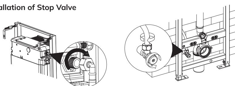
Connect the Flexible Hose to the Stop Valve
