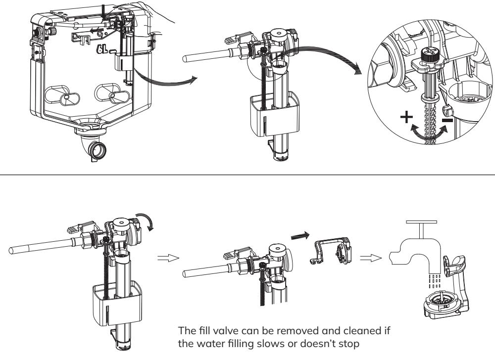
The fill valve can be removed and cleaned if the water filling slows or doesn't stop
