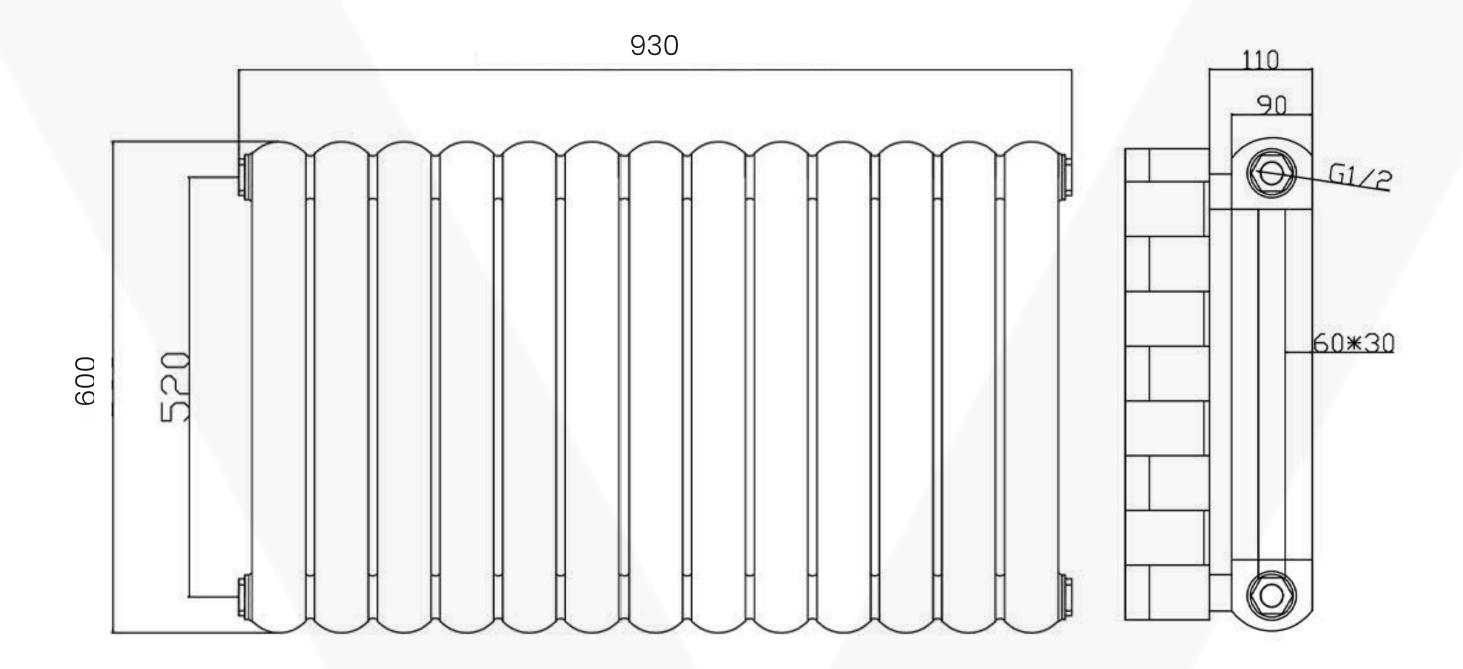
All Vaporo radiators are BOE and pipe centres are the radiator width plus 74mm.
