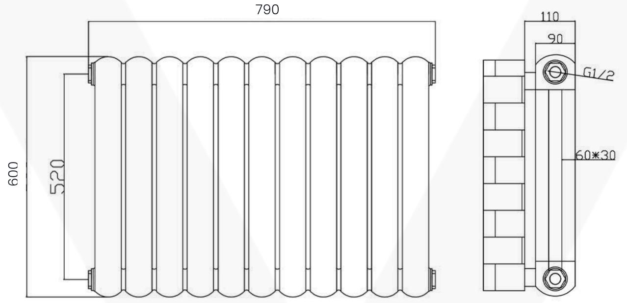
All Vaporo radiators are BOE and pipe centres are the radiator width plus 74mm.
