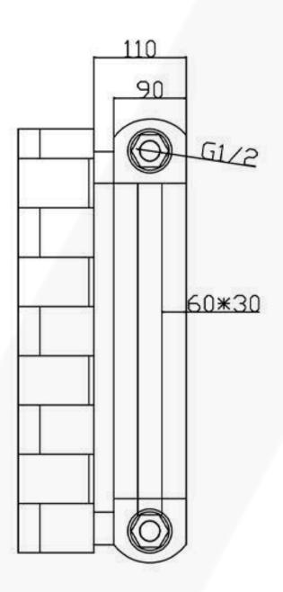
All Vaporo radiators are BOE and pipe centres are the radiator width plus 74mm.
