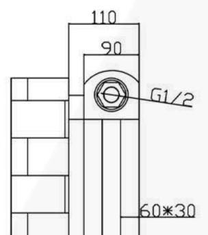
All Vaporo radiators are BOE and pipe centres are the radiator width plus 74mm.
